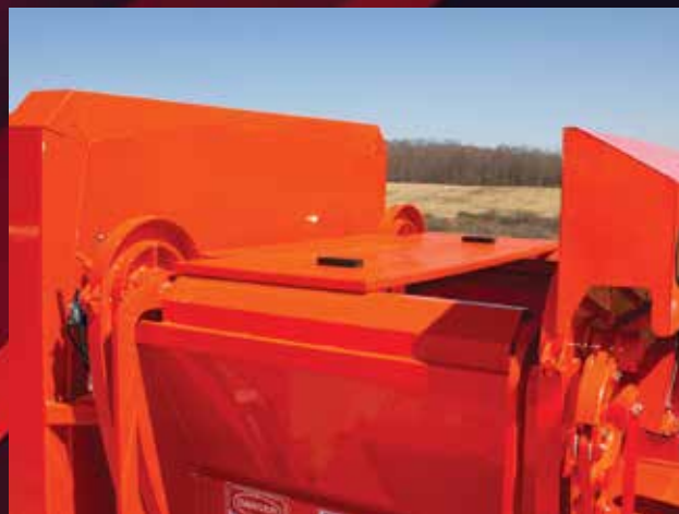
Debris Shroud Keeps Refuse In The Hopper
