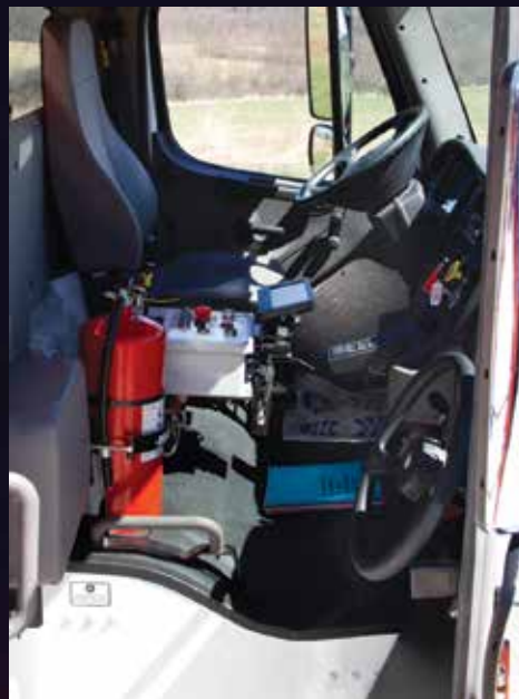
Optional Independent Side Loading With Dual Stand-Up Drive Cab Design
